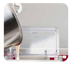
**Horizontal mixer** - The ingredients are poured into the hopper of the top cylinder. High rotation speed allows the dispersion of dry ingredients in the mix.
