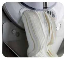
**Gelato extraction** - Once the cycle ends, the gelato is kept inside the machine at the right consistency; extraction is complete and fast due to the high rotation speed of the paddles and the wide opening for the gelato.
