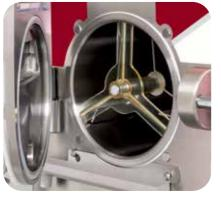
**Pasteurization** - Pressing the heating button will start the cycle, which can be adjusted up to 221°F/105°C. The control buttons are immediately interpretable; an acoustic/visual signal shows that the temperature has been reached.
