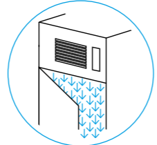
AIR CURTAIN TO REDUCE AMOUNT OF WARM AIR ENTERING WHEN DOOR IS OPENED
