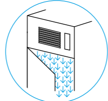
AIR CURTAIN TO REDUCE AMOUNT OF WARM AIR ENTERING WHEN DOOR IS OPENED
