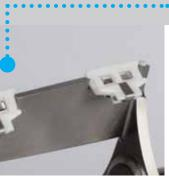
The scraping effect on the cylinder surface resulting in a extremely high heat rate efficiency as well as high energy saving is given by the strength of the materials the scrapers are made of, their special inclination on the touch point and the specific high-thrust spring.
