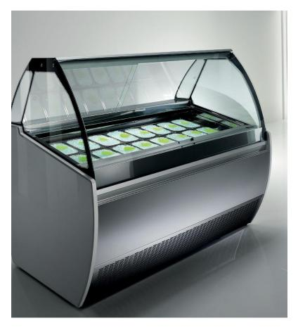
Features: Ventilated gelato and ice cream showcase with silver-anodized tubular aluminum, stainless steel and, polyurethane body construction, heated, tempered front glass with drop down opening, glass heated side, lamp holder with fluorescent lamps, rear closure with sliding doors or retractable blind as an option, internal compressor (remote as an option), electronic control unit on operator side, and reverse cycle defrost function.
