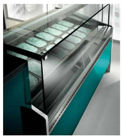
Features: Ventilated gelato and ice cream showcase with silver-anodized tubular aluminum, stainless steel and, polyurethane body construction, heated, tempered front glass with drop down opening, glass heated side, lamp holder with fluorescent lamps, rear closure with sliding doors or retractable blind as an option, internal compressor (remote as an option), electronic control unit on operator side. and reverse cycle defrost function.
